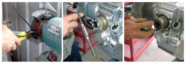
Clean the cap screw threads with a wire brush – make sure that there is no residual Loctite in the threads. Clean all threads with cleaning solvent (Loctite 7471 cleaner or Acetone) and dry.
