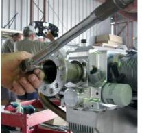
Apply a few drops of Loctite 620 to each screw hole, place the propeller flange extension on the hub and fit the 6 cap screws and washers.
