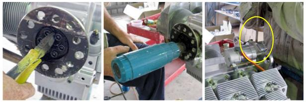
The universal flange is held in place by  $6 \ge 3/8$ " UNF Allen head cap screws, all of which will be reused.
